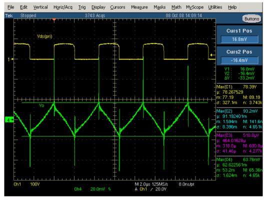
Figure 5. Output Voltage Ripple (37Vport, 5A)
