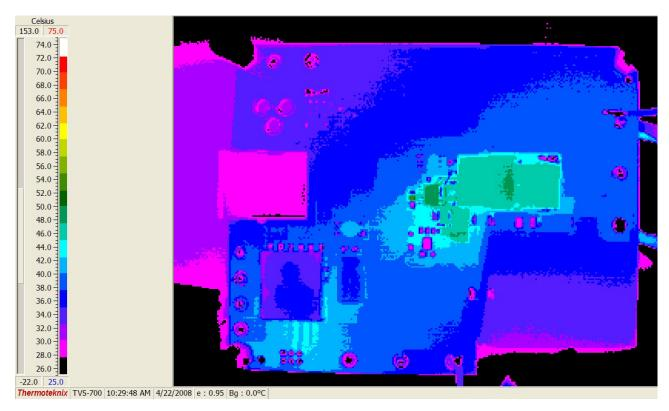
Figure 8. Temp Data (37Vport, 5A, Bottom)
