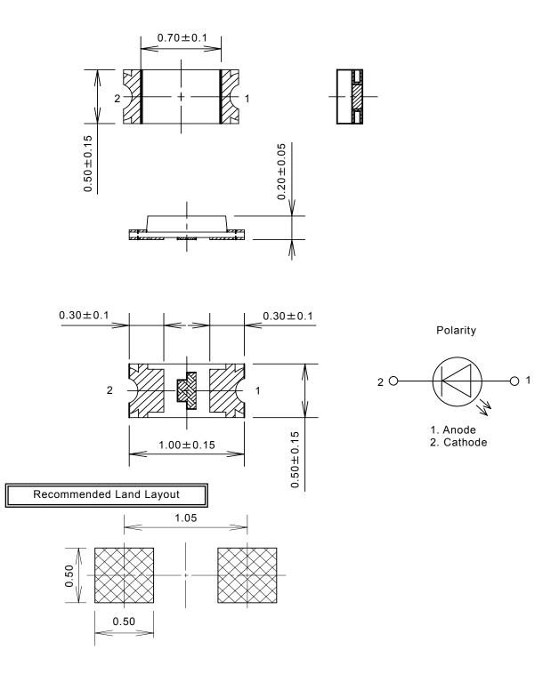
(Note1)Electrode projection is not included in the package dimensions. (Note2)About solder thickness, please examine the products yourself completely. (Recommended thickness : t=0.10 mm~0.15 mm)
