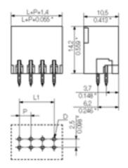
1729100000 S2L 3.5/36/180G3.5SN SW PCB plug-in connector, Male connectors, Soldered connection, Pitch: 3.50 mm, No. of poles: 36, 180°, Box 4032248040537 20 pc(s).
