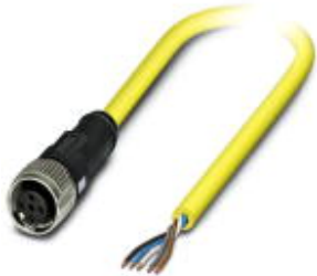
Sensor/Actuator cable, 5-position, TPE, yellow RAL 1021, free cable end, on Socket straight M12 SPEEDCON, A-coded, Cable length: 5 m
